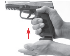
Insert the loaded magazine completely into the magazine well until it latches in place.
