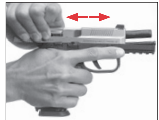
Pull the slide completely rearward and release it, allowing it to move forward freely.
